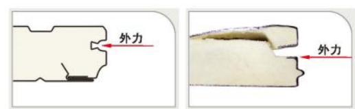
凹凸型安然无恙 Concave and convex panel is safe 传统中间接口板接口开裂 Traditional Model
