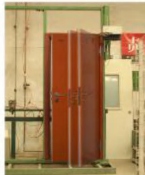
200,000 times in the fatigue test
