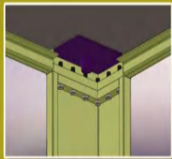
立柱与顶梁连接 The Corner post jointed with the top beam
