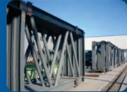
Pipe truss type structure
