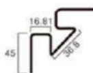
内角 Inside Corner Post(Ha 1) Length: 2.95m Pieces per carton: 16 Coverage per carton: 47.2m
