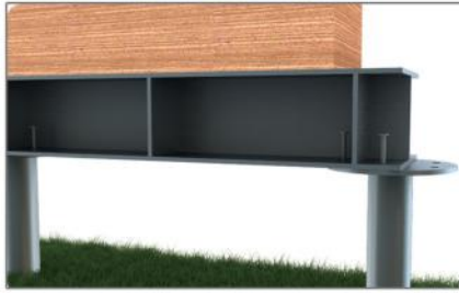
Light steel chassis support
