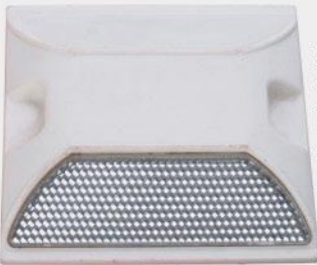
型号(model):LZL-DD-02 材料(material):塑料(plastic); PC反光片(PCreflective sheeting) 规格(specification):双面(double-side) 反光(reflective) 尺寸(size):100 × 100 × 20mm
